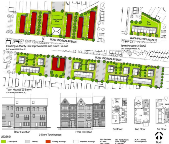
Architectural Design and Site Plan of Townhouse Development Concept Arranged Around a Common Green Space
